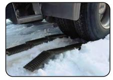
The short section is placed in line with the stuck tire with the traction side up. The bottom of the short section is smooth; allowing the tool to slide under the tire as the driver slowly accelerates.
